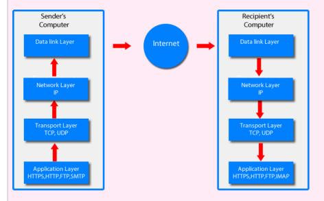
The **application layer** contains protocols associated to the particular application such as HTTP, HTTPS for web browsers, FTP for file transfer or SMTP and POP3 for email for instance. The application layer interacts with the user via appropriate application software (eg web browser / ftp client / email client).
