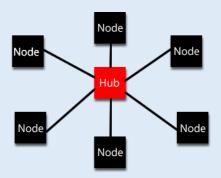
on one topology can behave as if is has been set up as another topology. For instance, a network that has physically been set up at a star topology can
